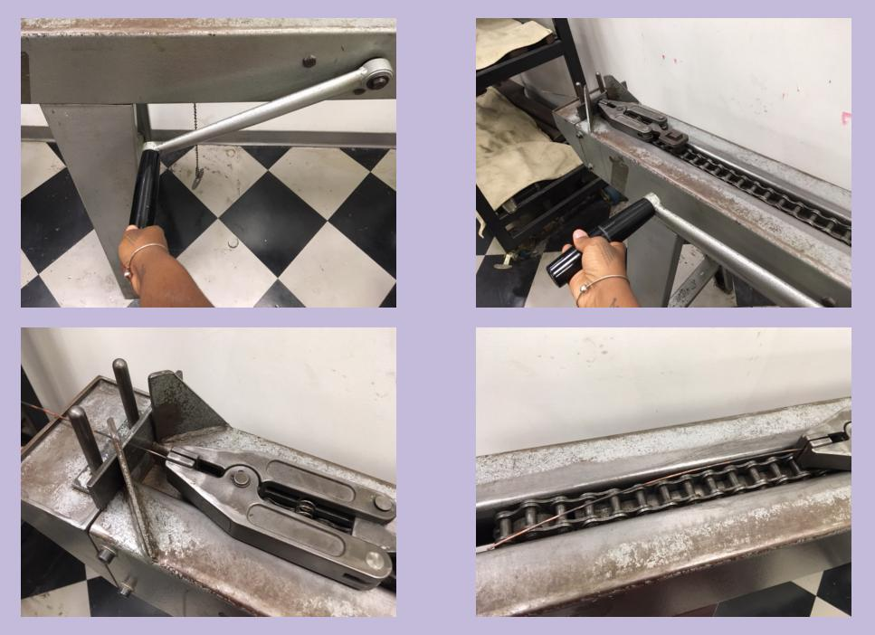
Use drawing bench handle to pull drawing tongs on mechanism. You will continue to rotate handle until the wire has been completely released from the draw plate.
