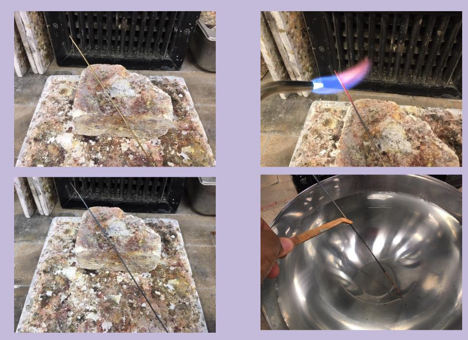
Once your wire is tapered, you can take it to the soldering station and anneal it. Be sure to anneal wire well or you can damage the draw plates because the wire can break away from drawing tongs/plates. After annealing you metal, you must quench your wire in water.
