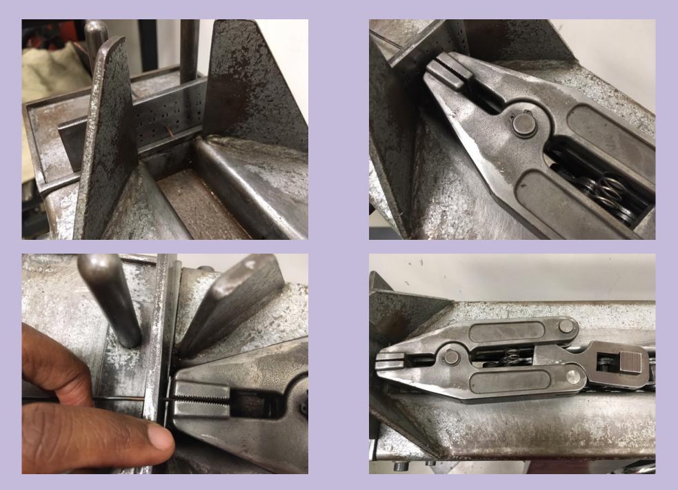
Place draw plate into the draw plate holder. Then place wire into the gauge size you want to draw your wire to. Use the drawing tongs to grip the tappered end of the wire.
