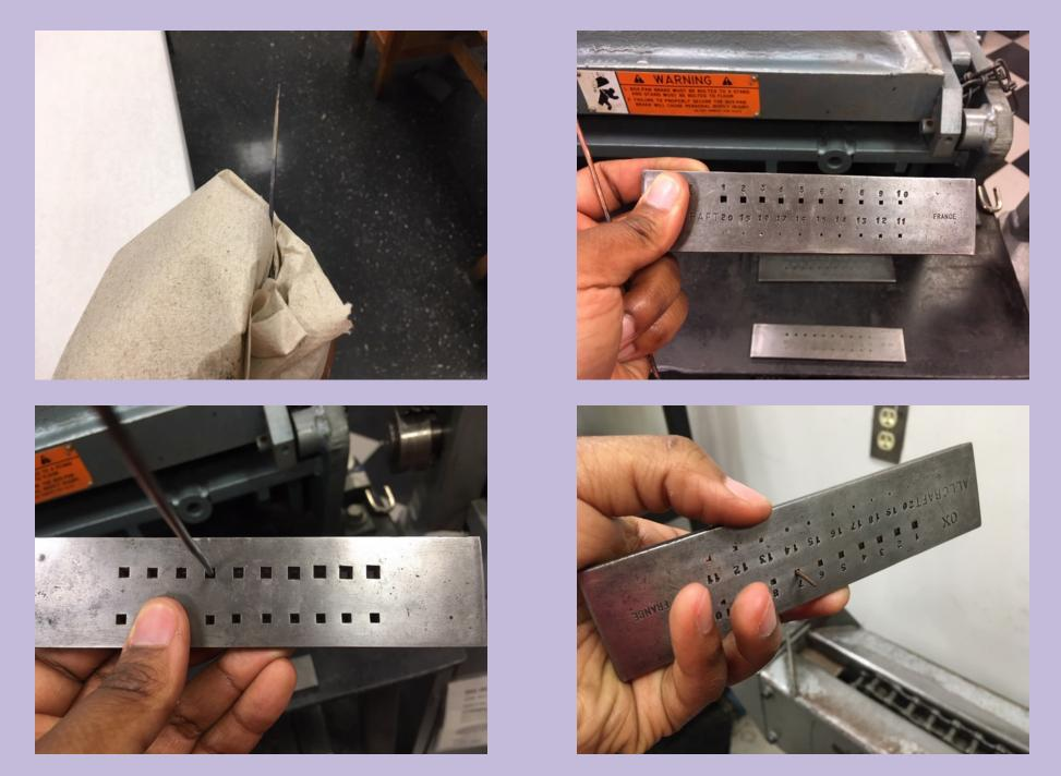
Be sure to dry your metal before putting it through the draw plate to prevent the plate from rusting. Once dry, choose the correct shape and size draw plate you want to use. Wire must always be inserted from the backside where you cannot see the guage size. Inserting the wire in the incorrect way can damage the draw plate and cause the wire to get jammed.
