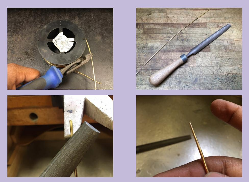
First choose a wire gauge that is closest to the guage you are trying to acheive using the draw plate. Once you have chosen your wire guage, you must prepare to taper it so that it can fit inside of the draw plate. To prepare your wire you can use a rough file until 10-15mm of your wire is tapered.
