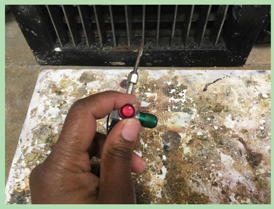
Put torch tip near ventilator to release the rest of the gas and oxygen from inside of both lines.
