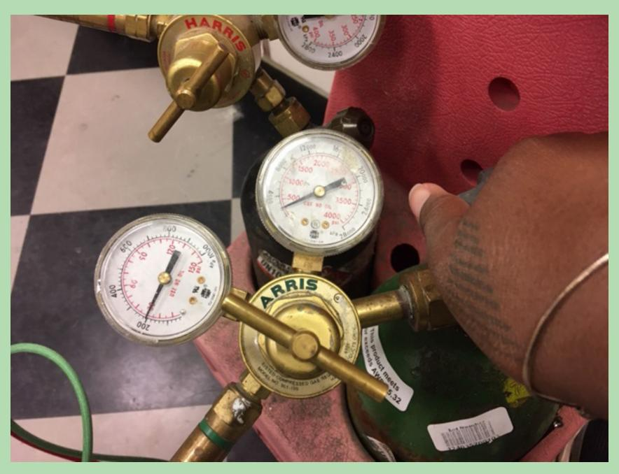
Turn valve to the right to shut off oxygen/close regulator. (Lefty Loosey Righty Tighty)
