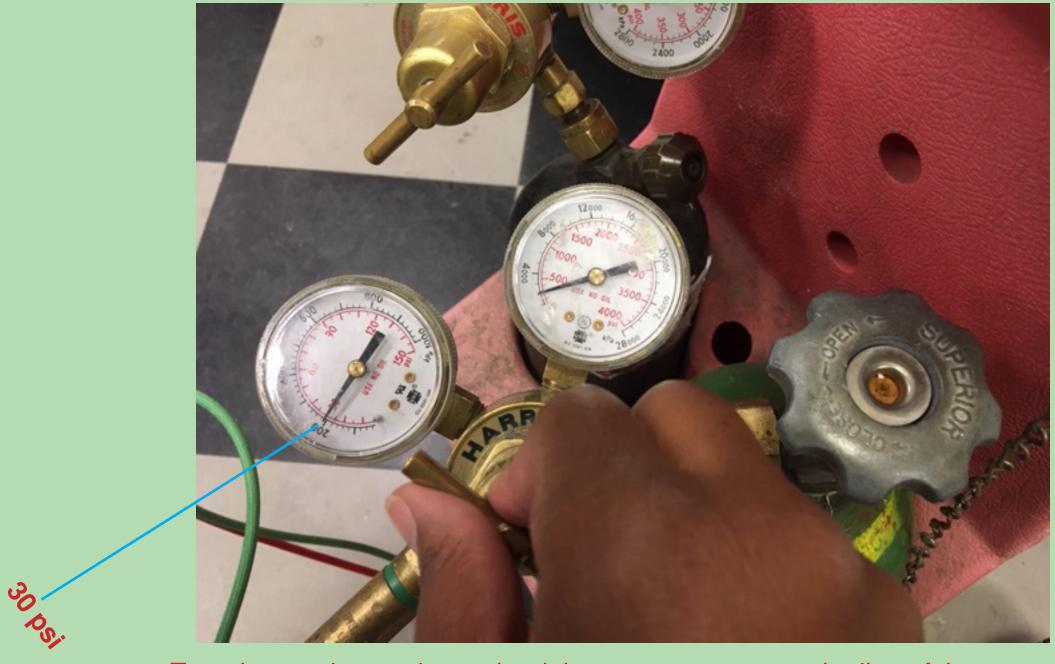
Turn the regulator valve to the right to put pressure on the line of the oxygen.
