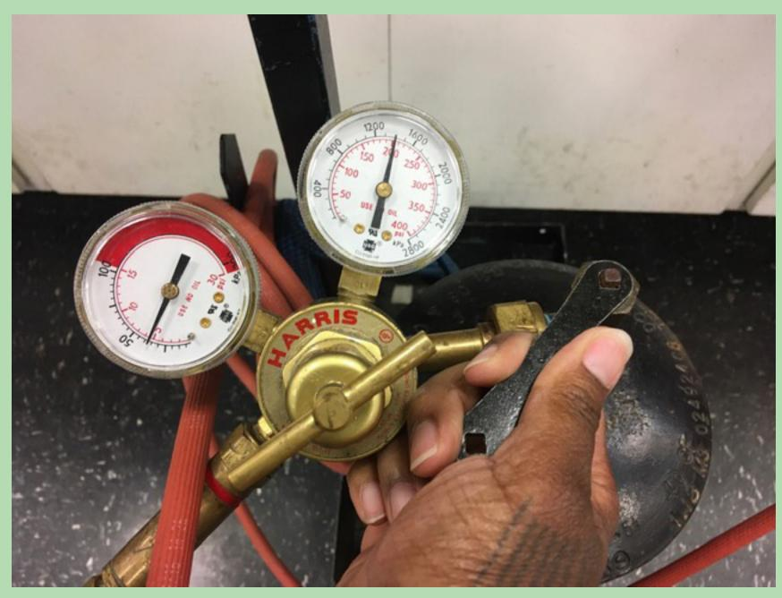
Turn tank key to the right to shut off gas/close regulator. (Lefty Loosey Righty Tighty)
