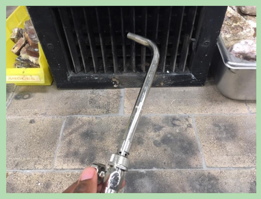
Put torch tip near ventilator to release the rest of the gas from inside of the line.
