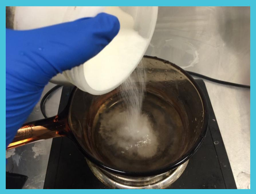
Place citric acid inside of the water. The amount needed is depended upon the amount of water used/size of piece.
