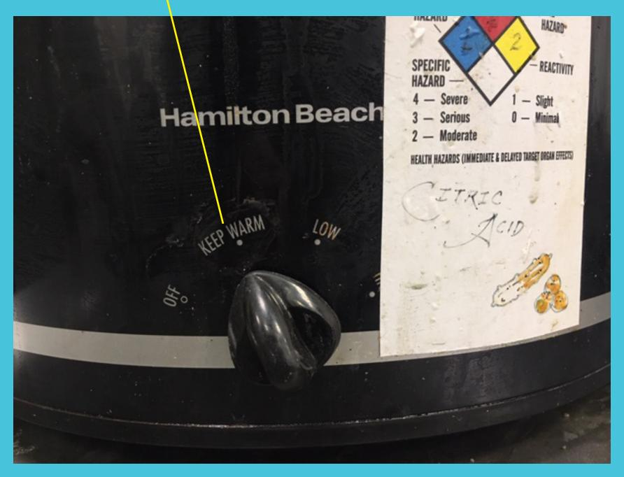
Always be sure that the pickle pot is set to keep warm. Setting the pickle pot to high could cause much harm and it does not speed up the process.
