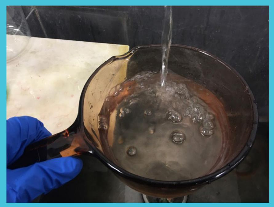
Put water inside of the glass bowl. The amount of water needed is depended upon the size of the piece. Pickle solution and oxygen beach/hydrogen peroxide should be measured in equal parts. (You can also use an electric water kettle to save time from heating the super pickle).
