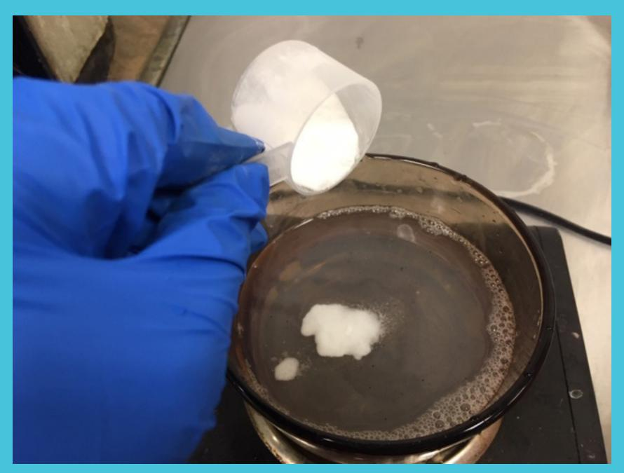
Once you are done super pickling, be sure to use baking soda to neutralize the solution before pouring it down the drain. While pouring soultion down the drain, be sure to run water to help keep sink area clean.
