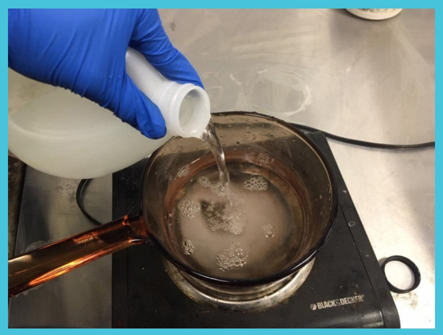
Pour an equal amount of oxygen bleach/hydrogen peroxide inside the glass bowl that already has the water/citric acid. Once both parts are mixed together, you can turn the hot plate on.
