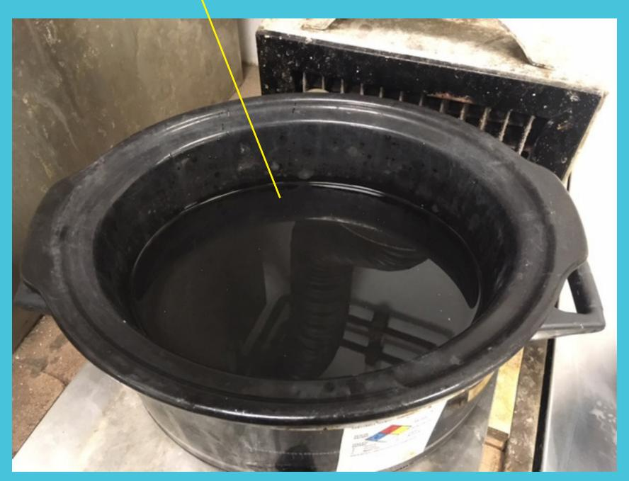
Fresh pickle is clear, however as it is continously used the color changes (this doesn't necessarily mean that the pickle needs to be changed).
