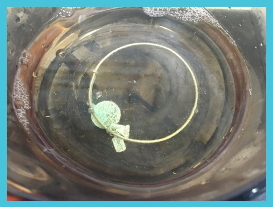
Heat allows the super pickle to perform at its best. Oxygen bleach allows the super pickle to work much faster than using hydrogen peroxide. Results should appear within minutes. (Remember to wear gloves and use copper tongs/practice all safety precautions).
