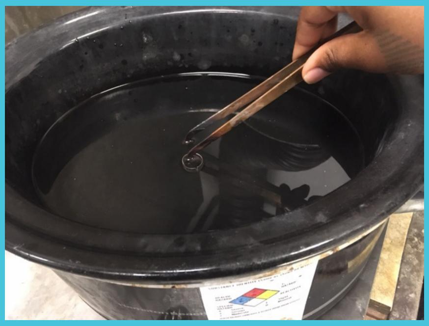
Be sure to use copper tongs when taking work out of the pickle pot. Never use steel tongs because it can contaminate the pickle. Never pick up piece with bare hands.
