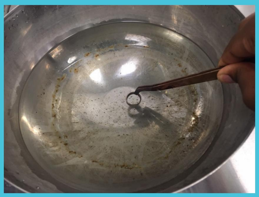
Immediately after taking piece out of the solution, place it inside of a steel quench bowl with water to remove acid.
